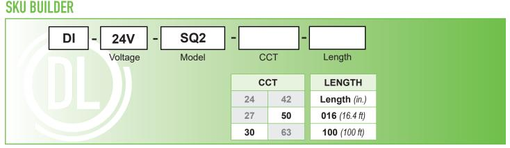
Example: DI-24V-SQ2-30-016= Diode LED, 24 Volt, SQUIGGLY<sup>™</sup> 200 LED Tape Light, 3000K CCT, 16.4'
